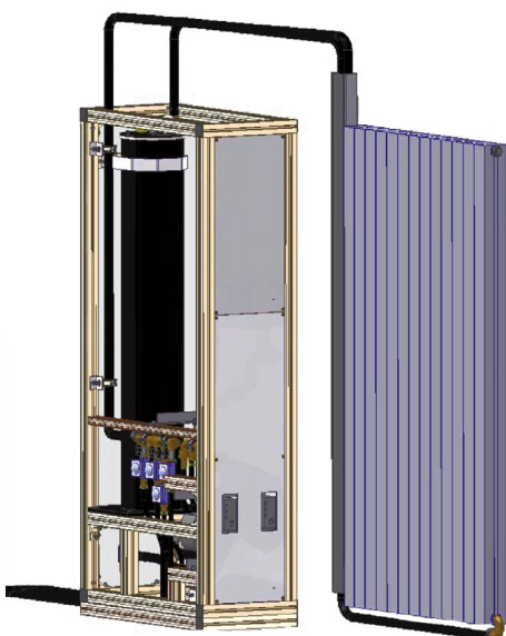
Pump unit and indoor cooler
